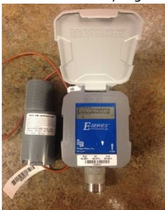
Photo 32: The new water meter
